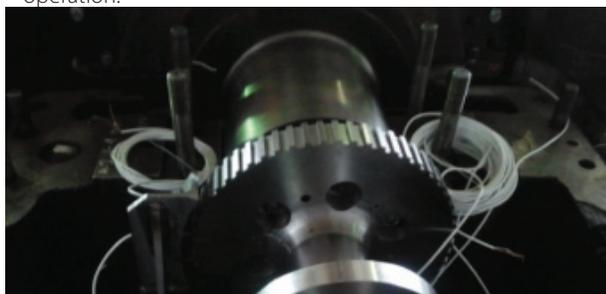
Figure 2- Turbine speed measuring assembly
